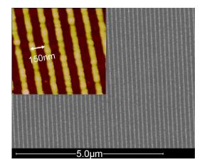
Fig. 4. Scanning electron microscope (SEM) image of the silver structured FSL. The dimensions are the same as shown in Fig. 3 inset. Inset: a zoom-in atomic force microscope (AFM) image shows the grating height is also quite uniform. The ridge width in AFM image is little bit larger than that in SEM image due to the finite size of the AFM tip.
